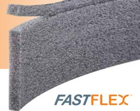
Fastflex<sup>TM</sup> is a closed-cell polyethylene foam expansion joint filler used in concrete construction. The convenient tear-off strip incorporated into the product makes it easy to create a void when using cold-applied sealants. Fastflex is particularly ideal for isolation joints accommodating different horizontal and vertical movement between the pavement and a structure.
